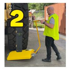
Lift the chock onto its front wheel and bring close to the tyre. Bring the back of the chock around into position.
