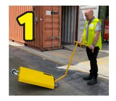
To move into position, pull the handle down, levering the chock onto its back wheels.
