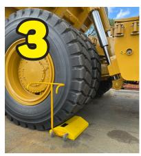
When chocks on both sides of the wheel are in position correctly, the truck is secured.
