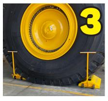
When chocks on both sides of the wheel are in position correctly, the truck is secured.
