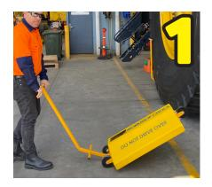
To move into position, use the foot bar to help pull the handle down, levering the chock onto its back wheels.
