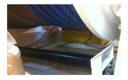
» Slack rope hoist drum trip roller system
